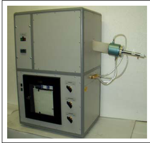
Figure 3: Gas evolution tester employed by Zhang et al. [27]. Dietert et al. [25] and Moore and Mason [26] employed similar devices to study gas evolution from bonded sand. The illustration was obtained from Reference [31].
